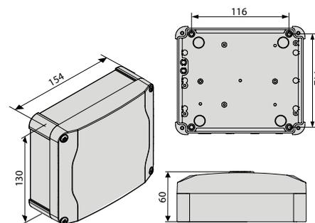
Ricevente radio esterna in quadro, 433 MHz, rolling code.
